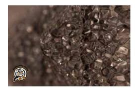
Its characteristic structure makes it suitable for all those applications where high soundproofing or thermal insulation is required, such as in firing ranges.
